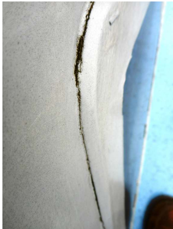
Fig 24. Slight movement at coachroof window.
