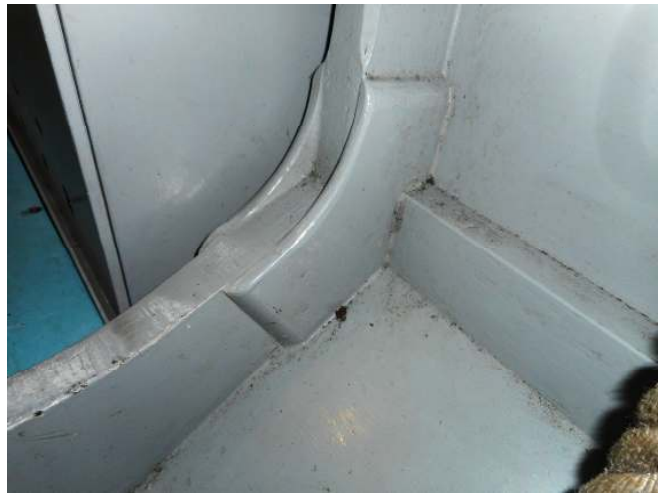
Fig 15 (below). Detail of reinforcement over chine.
