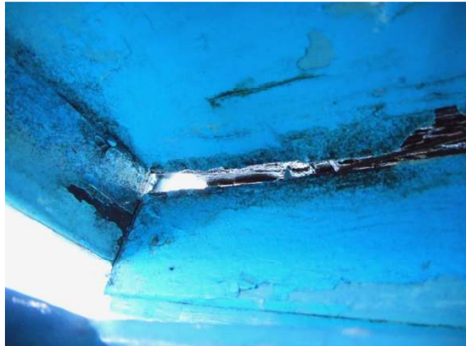
Fig 23. Deterioration in starboard aft hatch.
