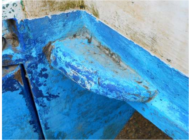
Fig 7. Detail of root of skeg / sternpost, showing reinforcing quadrant.
