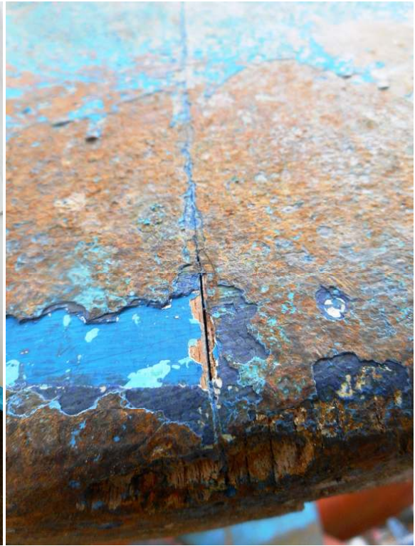
Fig 36. Detail of open seam on port rudder blade.
