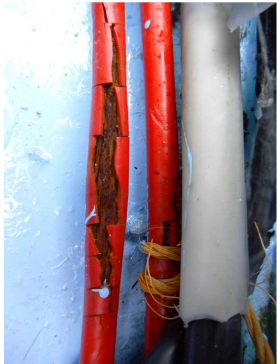
Fig 42. Corrosion in throttle and gear control cables.
