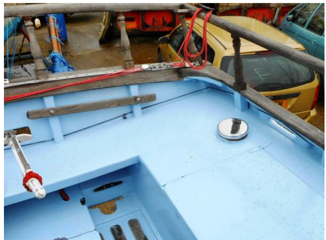
Fig 31. Cleat and fairlead, port quarter.
