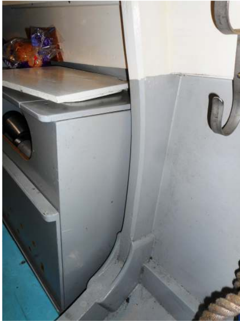
Fig 14 (left). Example of frame in port hull.
