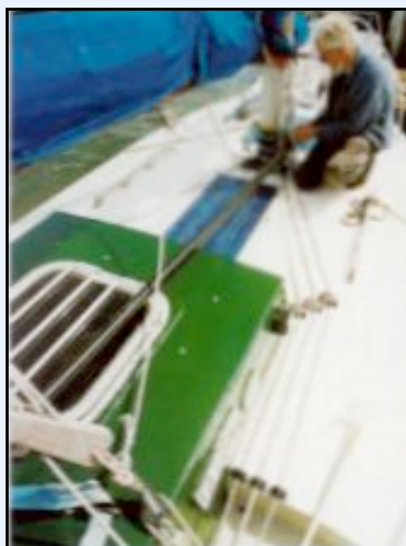
All the junk rig control lines are led aft to a set of turning blocks on the stern and then back inside the cabin to the winches.
