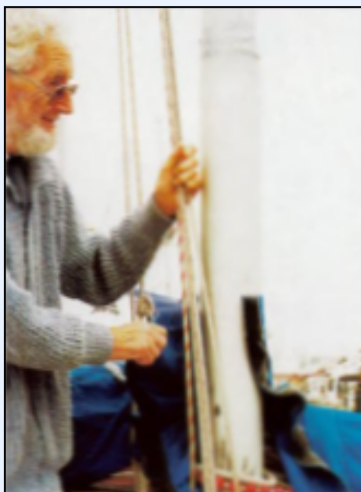
The mast could be pivoted back. Its special hinged joint is covered by a long metal sleeve
