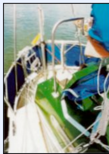
All the junk rig control lines are led aft to a set of turning blocks on the stern and then back inside the cabin to the winches.
