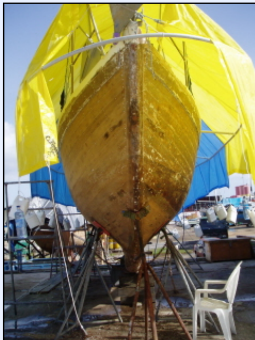
Cladding Speedwell in fibreglass
