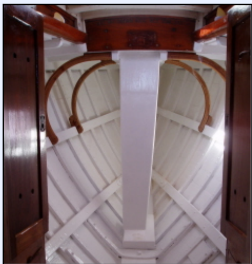
Tabernacle compression post and four laminated teak knees -note 'cutaway' on starboard side to make forward access easier
