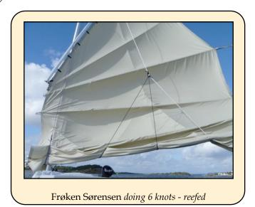
Yard and battens are also aluminium. The sail is made from Odyssey III and has 8% camber. Set up with Arne's usual throat-hauling parrel and Hong Kong parrels, the sail sets beautifully and performs well.
