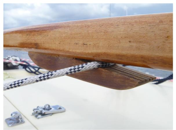
Ingeborg's hardwood brake with only 8° notch, jams the line firmly, to cope with the higher tiller forces.
