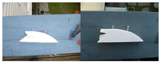
The core of Frøken Sørensen's tiller brake, before and after modification to a narrower notch.
