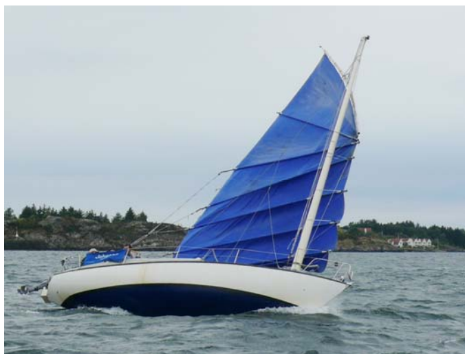
.. Johanna's mast, LAP=9.6m, diameter at deck level=25cm. and at mast top 10cm The "sail area" of the mast is thus close to 1.7m 2 - quite a drag factor on the sb. tack...
