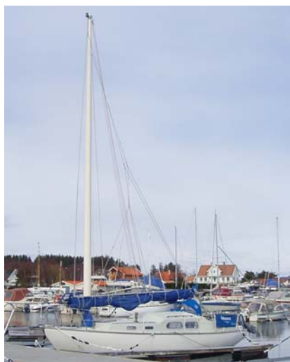
.. Johanna's mast, LAP=9.6m, diameter at deck level=25cm. and at mast top 10cm The "sail area" of the mast is thus close to 1.7m 2 - quite a drag factor on the sb. tack...
