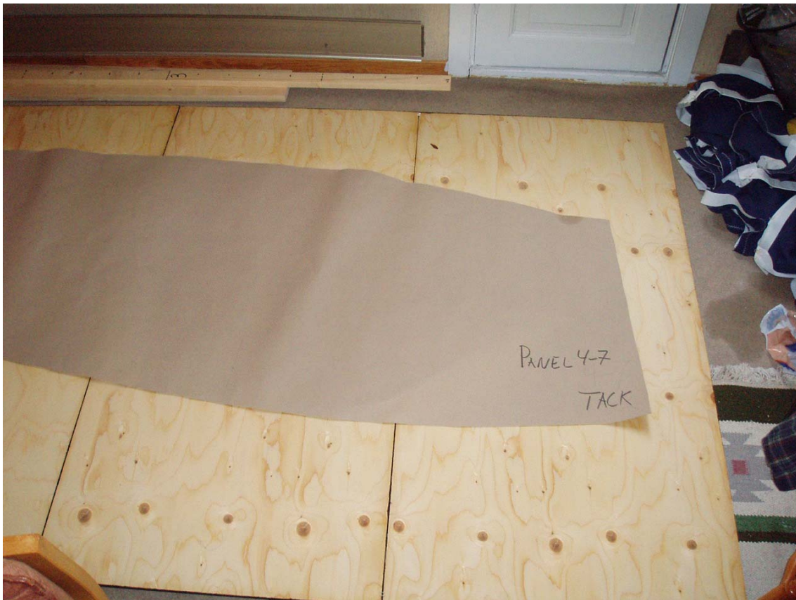
The paper template for Broremann's lower panels. Note the rounding along battens; the barrel shape.
