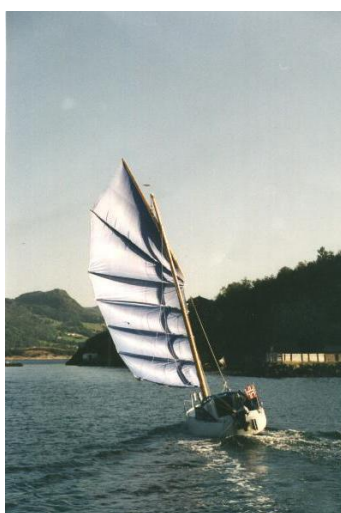
1994, new sail with cambered panels
