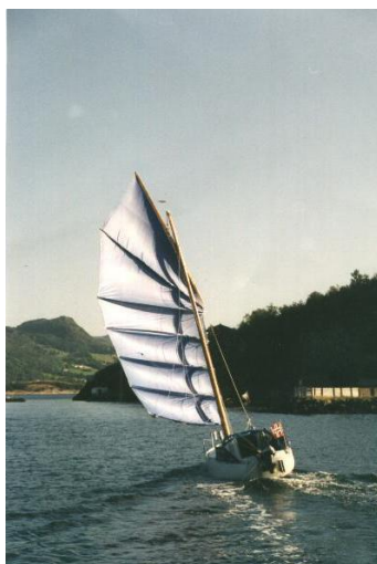
1994, new sail with cambered panels
