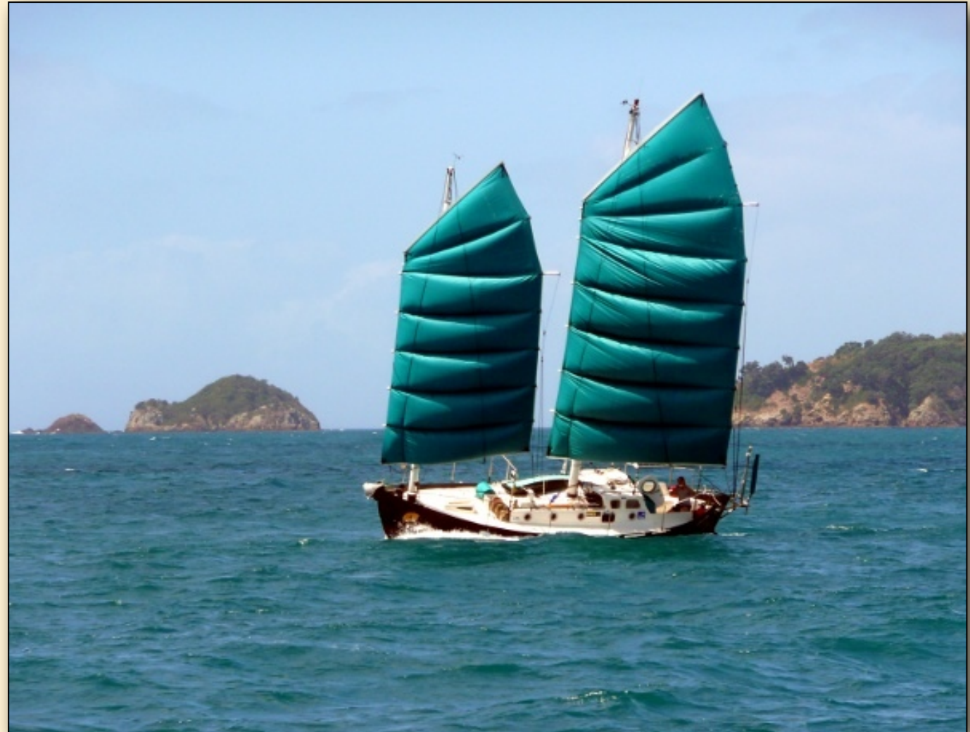
La Chica, with her cambered panel sails made from Mustang fabric
