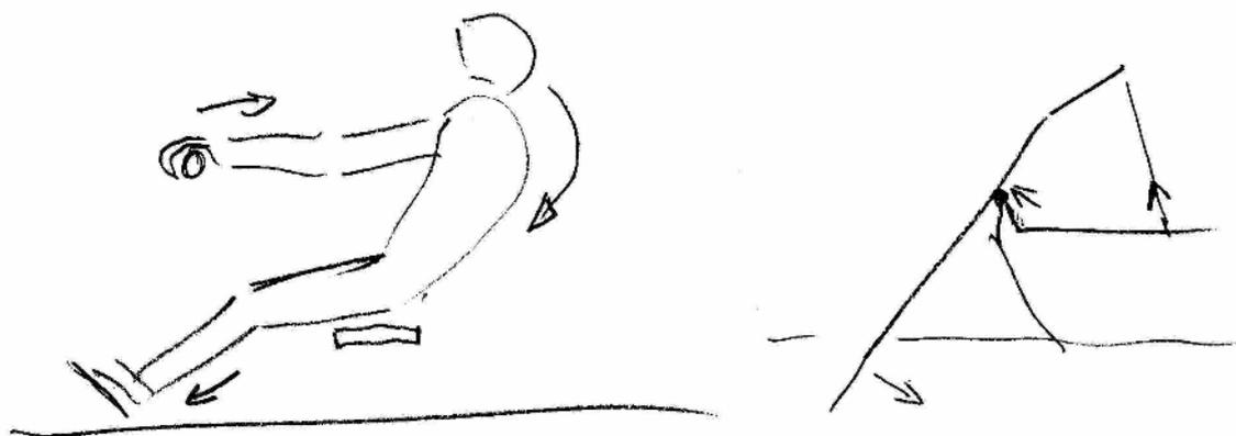
Comparing the hydrodynamic performance of the oar to the yuloh is similar to comparing the paddle steamer to a propeller driven vessel, and it is well documented that the propeller is more efficient than the paddle wheel. This would suggest that the basic action of using the yuloh should require significantly less effort than using oars to produce the same work.
