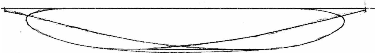
The diagram above is simply the Clark Y section and mirror image superimposed in an effort to draw a two way section to give a downward force. (The only lifting foil that requires a leading edge at both ends that easily comes to mind is the Frisbee, which might be a good starting point). A compromise would have to be reached to combine hydrodynamic efficiency and mechanical strength. Ease of manufacture must also be considered.
