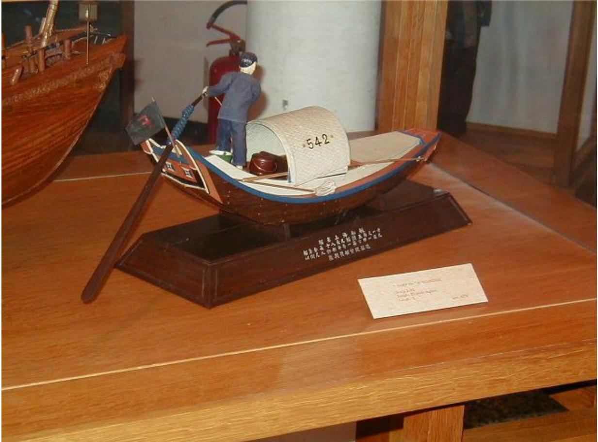
The photographs of the harbour sampans show the elevated position of the yuloher and the raised transom to support the fulcrum. It is not a large heavy vessel, so the yuloh does not extend to above head height.
