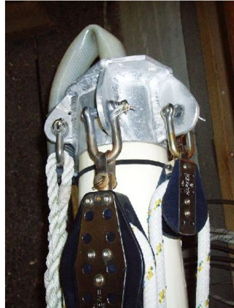
Johanna's masthead (aluminium). From left to right: Mastlift, halyard - and halyard; I use 2 blocks. Note plastic hose on top which covers the lantern wire. For size referenc; the lines are 10mm
