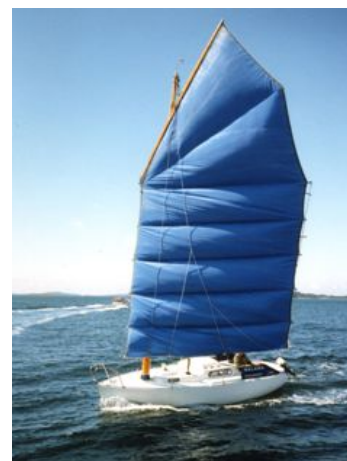
1999, with taller mast and 7 panels.
