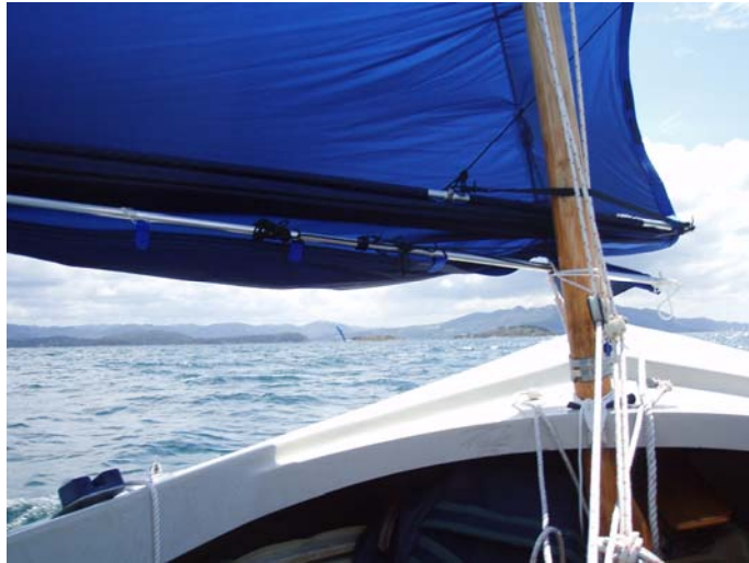
Broreman with one reef, showing the moderate negative stagger
