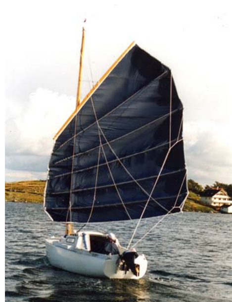
..Malena's fanned sail in 1992; the boom and yard taken from the original sail, are shorter than the battens...
