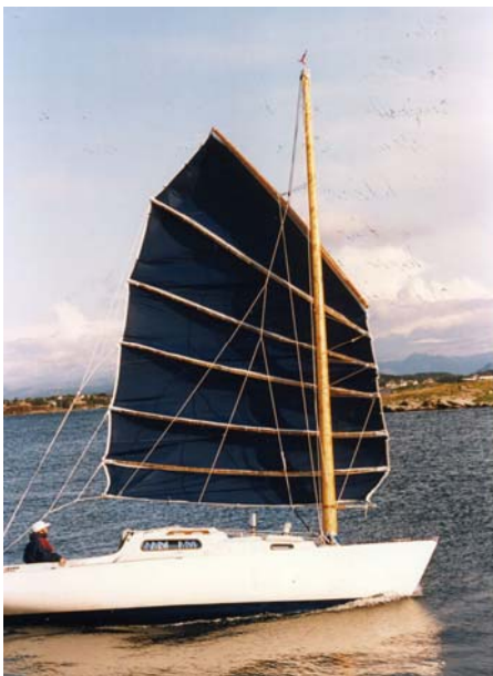
..Malena's fanned sail in 1992; the boom and yard taken from the original sail, are shorter than the battens...
